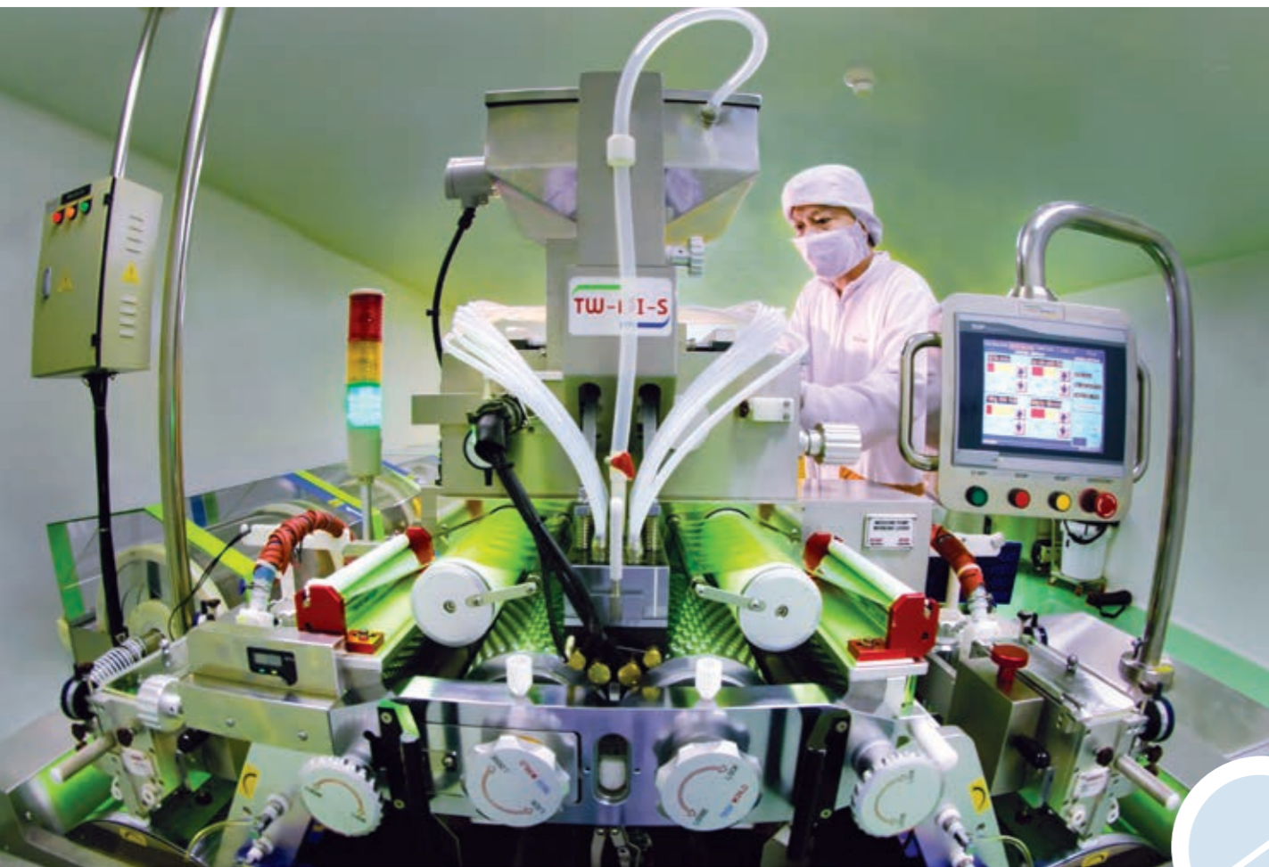
A machine producing soft capsules at DHG Pharma.
