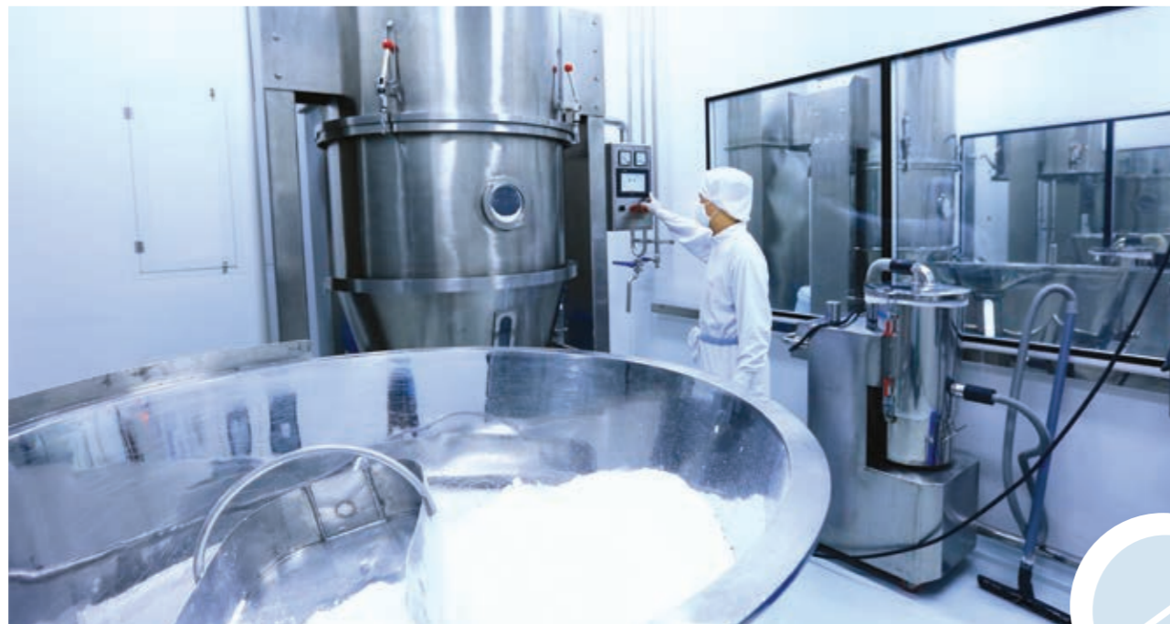
A fluidized bed dryer at the plant of DHG Pharma
